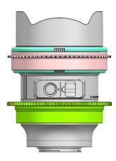
The tightness between the both gears and the lens can be adjusted by removing or adding rubber grips on either sides of the plastic C-ring, spare rubber grips are included in the package.
