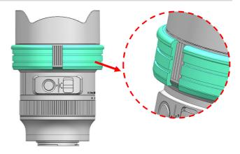
Insert the plastic C-ring for focus gear as shown and place it over the lens
