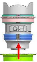
Insert the SLE1424-Z zoom gear on the plastic C-ring until it reaches the flange of the plastic C-ring.
