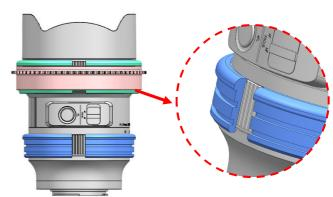
3. Insert the plastic C-ring for zoom gear as shown and place it over the lens
