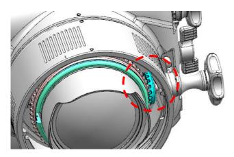
The SLE1424-F Focus gear can be controlled through the focus knob of #21250 N120 Extension Ring 50 with Focus Knob.
